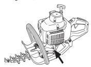
**CAUTION!** The gear housing must not be filled completely with grease. The grease expands as the machine heats up during operation. If the gear housing was completely filled with grease it could damage the seals and lead to leakage of grease.
